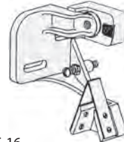
B037AC-16 Lower Carbide Block & Cleaner Holder Assembly with Steel Blade Cleaner
