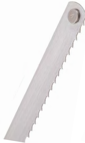
NEW SB30002 Toothe Edge 4 TPI 5/8 x .022 x 17 5/8"
