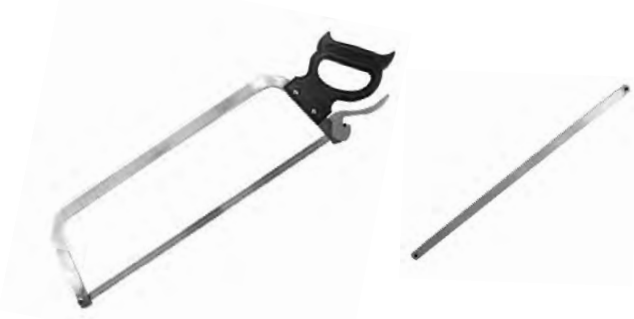
NEW HB12-20 Hand Saw Blade 20" Long x 1/2" wide .025" thick 10 Teeth /Inch
