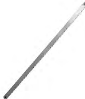
NEW HB58-20 Hand Saw Blade 20" Long x 5/8" wide .025" thick 10 Teeth /Inch
